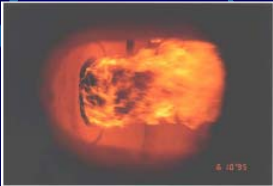
Conventional and flameless combustion of heavy fuel oil. Prototype swirl burner for heavy fuel oil - power 100 kW e . Oxidizer: standard atmospheric air (21% O 2 ) at 250°C.
